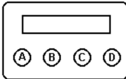
When you get to the end of the menu it will start over from the beginning. Buttons C and D adjust the values. Button C decreases the value and Button D increases the value. All changes are made immediately, what you see on the screen is what the Magic Box is running at. All adjustments can be made with the engine stopped or running.
