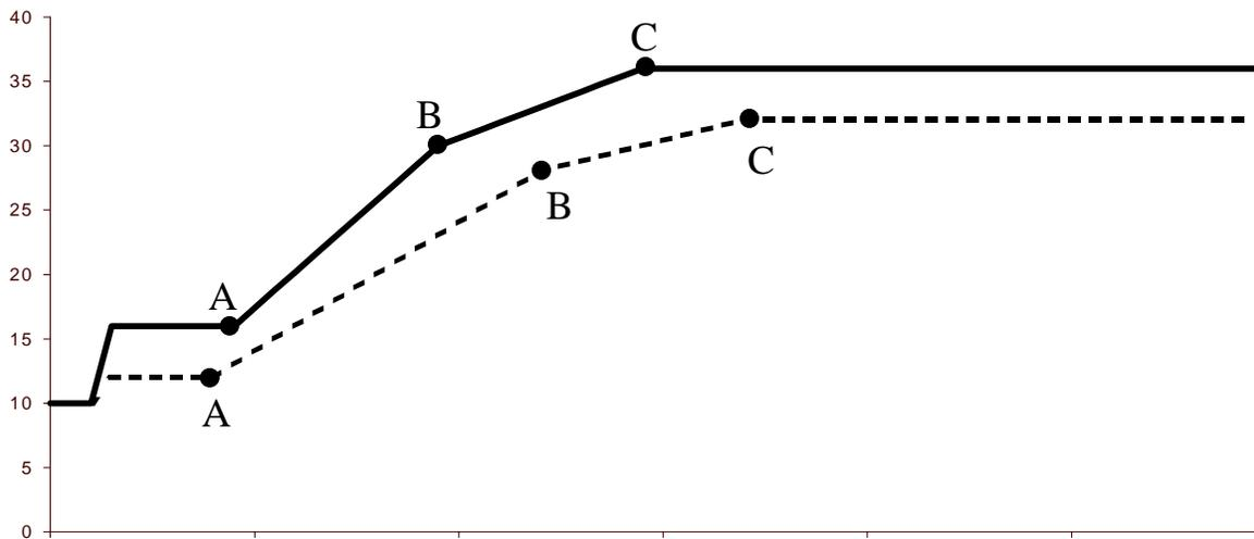
The advance curve is set with three plot points; initial advance (A), mid advance (B), and max advance (C). Above is pictured the two default curves. The dotted line is the default street curve and the solid line is the default strip curve. Any time the computer is disconnected from the battery it will revert back to the default settings.
